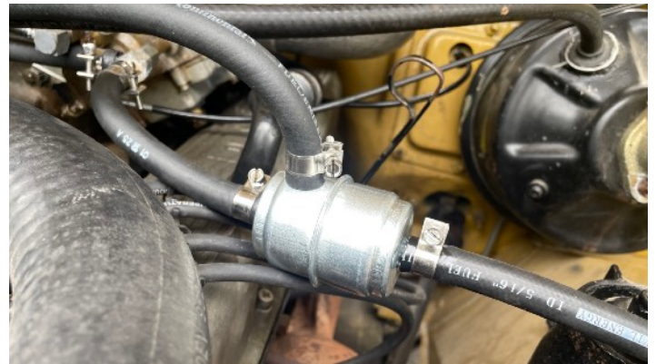
Separator filter in slightly modified form: FRAM G3499
