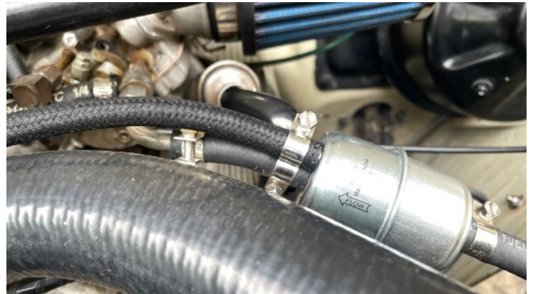
Vapor trap with fuel filter - Purolator F21117. Note: Limited space between the two outlets.
